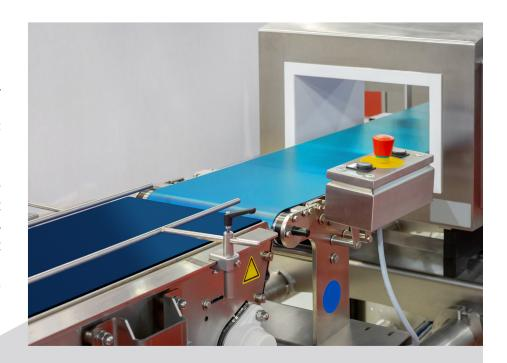
Agilext offers a line of conveyor belting that uses a highly metal detectable, fine, stainless steel powder additive to identify plastic contamination and prevent plastic contaminated foods from reaching consumers. This additive imparts a gray color into the belt. Colorants can, also, be used to produce darker colored belts like blue, green and purple. It also provides X-ray contrast.
